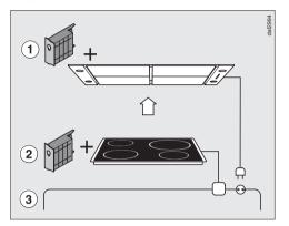
Communication module XKM 2000 DA ①, available as an optional extra, enables the operation of the cooker hood to be automatically controlled by the operating status of a Miele electric hob with onset controls.
